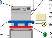
Single block IP 55 electrical cubicle made in mild steel or stainless steel including the speed variators, transformer, 24V power supply, the relays, the connecting terminal as well as the circuit breaker and the emergency stop
