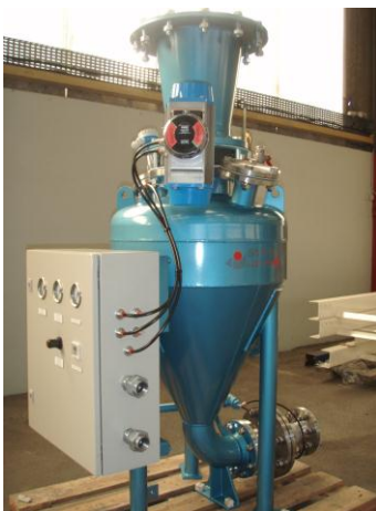
Control command cubicle
