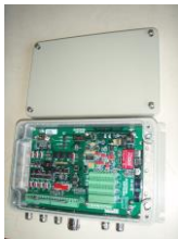
Digital signal processing unit
